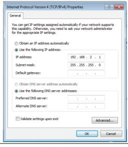
Click 'Use the following IP address', and then input '192.168.2.1' in 'IP address' and '255.255.255.0' in Subnet mask', just like shown on the left.
